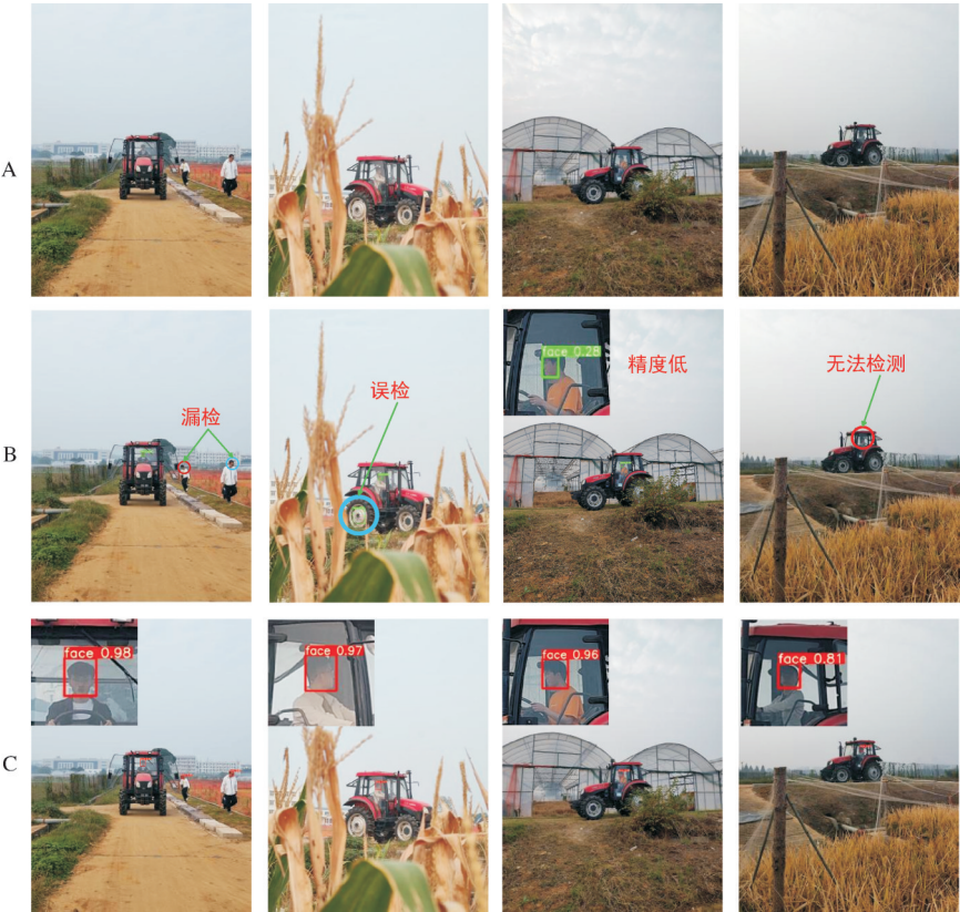
A:原图 Original; B:YOLOv7 检测结果 Detection results of the original YOLOv7; C: YOLO-SOD 检测结果 Detection results of the YOLO-SOD.
