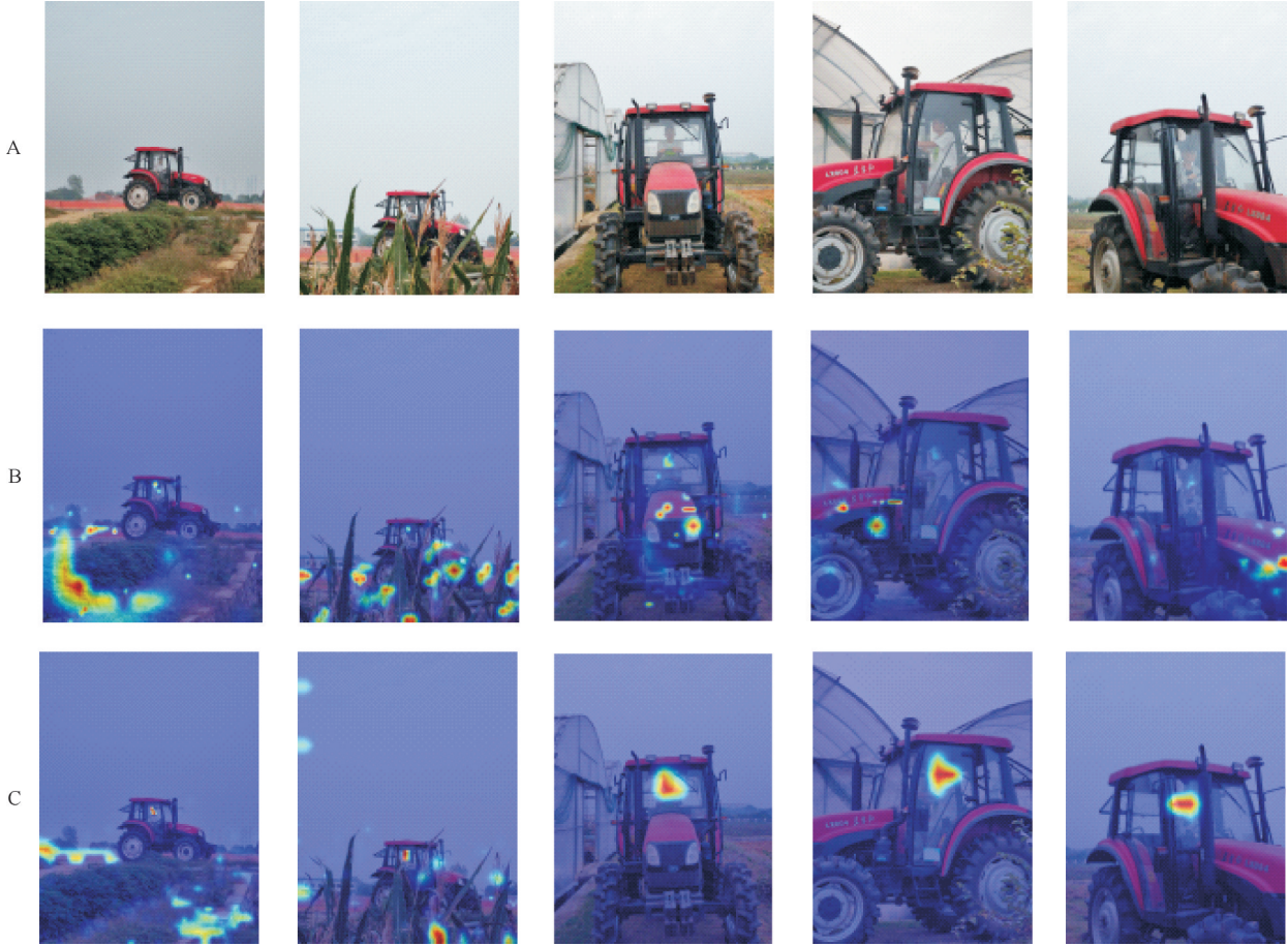
A:原图 Original picture;B:原始 YOLOv7 检测结果 Detection results of the original YOLOv7;C:改进后 YOLO-SOD 检测结果 Detection results of the improved YOLO-SOD model.
