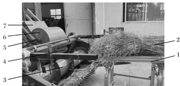
1. 输送带 Conveyor belt; 2. 油菜植株 Rape plant; 3. 割台喂入搅龙 Header feeding auger; 4. 喂入辊 Feeding drum; 5. 切碎滚筒 Shredding drum; 6. 罩壳 Cover; 7. 出料口 Material export.
