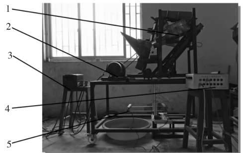
1.排种器 Seed-metering device; 2.三相交流减速电机 Three-phase AC motor; 3.易驱变频器 Frequency converter; 4.检测系统 Detecting system; 5.对射式光栅传感器 Grating sensor.
