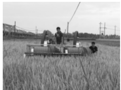
图 5 双割台双滚筒全履带式再生稻收割机 Fig.5 Tracked combine for ratoon rice with double-headers and double-threshing cylinders
