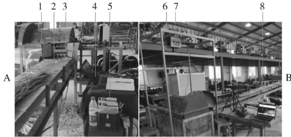
A: 顶盖受力采集 Force collection of cover; B: 高速摄影 High speed photography; 1. 传感器 Sensor; 2. 输送带 Conveyor belt; 3. 强制喂入轮 Forced feed wheel; 4. 笔记本电脑 a Computer a; 5. 变频器组 Inverter group; 6. 高速摄影台架 High-speed photographic stand; 7. 高速摄影仪 High-speed camera; 8. 笔记本电脑 b Computer b.
