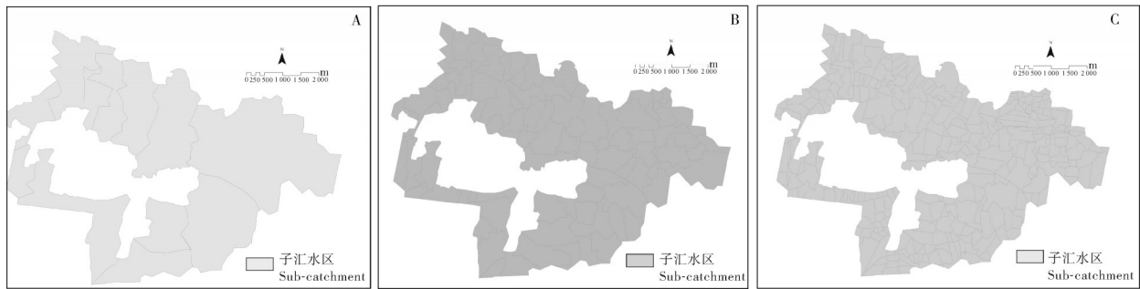
A:南湖汇水区划分 South Lake catchment area; B:基于水文分析及高程数据的子汇水区划分 Sub-catchment delineation based on hydrological analysis and elevation data; C:基于泰森多边形调整后的子汇水区划分 Adjusted sub-catchment delineation based on Tyson polygons.
