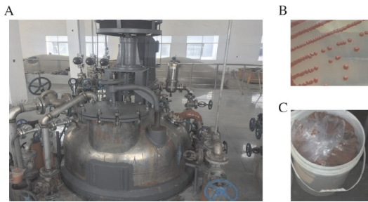
图3 酿酒酵母高产番茄红素中试放大至6000 L规模 Fig.3 High lycopene production from Saccharomyces cerevisiae scaled up to 6000 L
