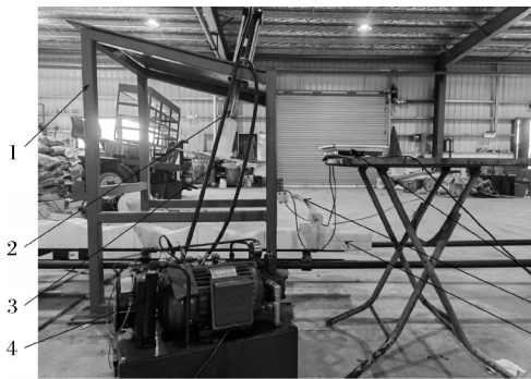
1. 试验台架 Test bench; 2. 液压油缸 Hydraulic cylinder; 3. 切割器 Cutter; 4. 液压站 Imitation ground mechanism; 5. 工控系统 Industrial control system; 6. 仿形机构 Imitation mechanism; 7. 仿地面机构 Imitation ground mechanism.
