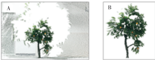
A: 分割前点云 Point cloud before segmentation; B: 分割后点云 Point cloud after segmentation.
