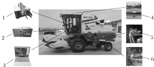
1.北斗RTK移动站Beidou RTK mobile station;2.导航控制箱 Navigation control box;3.工控电脑 Industrial control computer;4.北斗定位接收天线 Beidou positioning receiving antenna;5.电液比例阀组 Electro-hydraulic proportional valve set;6.角度传感器 Angle sensors.
