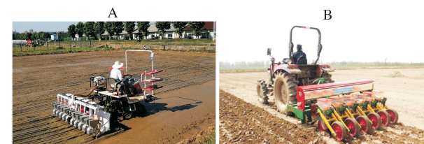
A: 机械化水直播 Mechanized rice water direct seeding; B: 机械化旱直播 Mechanized rice drought direct seeding.
