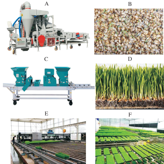
A:种子精选机 Seed cleaner; B:水稻种子催芽 Prompt germination of rice seeds; C:2BPX-800X 水稻秧盘播种机 2BPX-800X rice tray planter; D:水稻秧苗 Rice seedlings; E:水稻秧盘输送机 Rice tray conveyor; F:水稻秧盘 Rice seedling tray.
