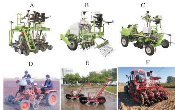
A: Monoseed DT 小区单粒播种机 Monoseed DT precision spaced planter; B: Plotseed S 轻型小区条播播种机 Plotseed S light plot seeder; C: Seed Pro 360 小区单粒播种机 Seed Pro 360 precision spaced planter; D: XBJ-150 型自走式小区播种机 XBJ-150 self-driving plot seeder; E: 2BZXJ-1 手扶式小区育种播种机 2BZXJ-1 Walking type plot breeding; F: 全自动化小区精量播种机 Fully automatic precision seeder.
