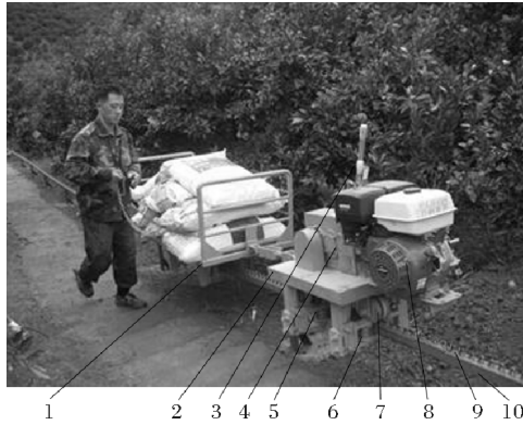
1.拖车 Trailer; 2.主车 Mail transporter; 3.刹车系统 Brake system; 4.传动系统 Transmission system; 5.驱动轮 Driving wheel; 6.夹紧轮 Clamping wheel; 7.导向轮 Guiding wheel; 8.动力系统 Power system; 9.齿条 Rack; 10.轨道 Rail.
