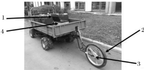
1.信号采集计算机 Signal collecting computer; 2.五轮仪 Fifth wheel instrument; 3.振动传感器位置 The situation of the vibration sensor; 4.速度显示器 Speed monitor.
