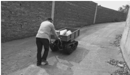
图 11 双履带运输车负重爬坡试验 Fig.11 Double track truck load climbing test
