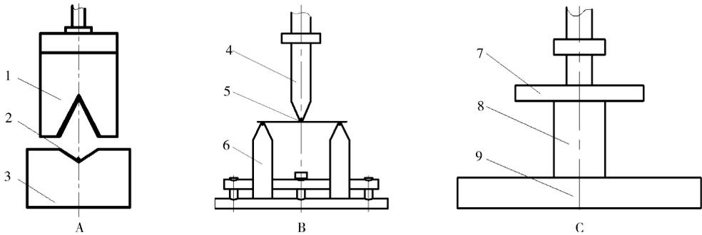
A. 剪切试验 Shearing test; B. 弯曲试验 Bending test; C. 压缩试验 Compression test; 1: 刀具 Tool; 2: 试样 Specimen; 3: 定位块 Fixed support; 4: 压头 Loading head; 5: 试样 Specimen; 6: 两端支座 Fixed 2 point-supports; 7: 压头 Loading head; 8: 试样 Specimen; 9: 底座 Base.
