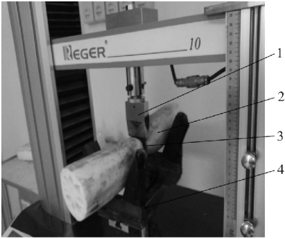
1.压头 Indenter; 2.莲藕 Lotus root; 3.藕节 Joints of lotus root; 4.支座 Adminiculum.
