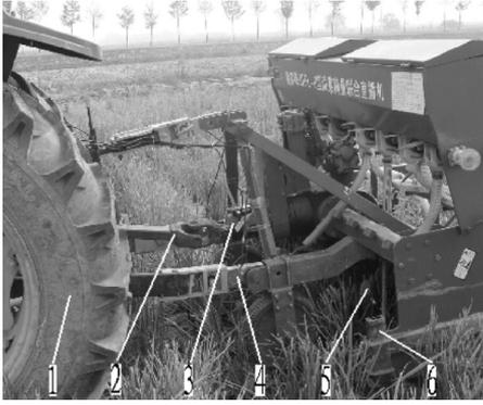
1.东方红-LX854 拖拉机 Tractor LX854 of Dongfanghong; 2.农用万向节 Agricultural universal joint; 3.转矩转速传感器 Torque-rotary speed sensor; 4.拉压力传感器 Force sensor; 5.种床整备装置 Device for seedbed prepared; 6.开畦沟犁型 Ditch plow.
