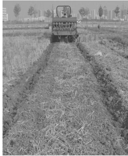
A: 深浅旋组合式种床整备装置作业效果 Performance of deep-shallow rotary tillage device; B: 作业幅宽全旋耕装置作业效果 Performance of full rotary tillage device.
